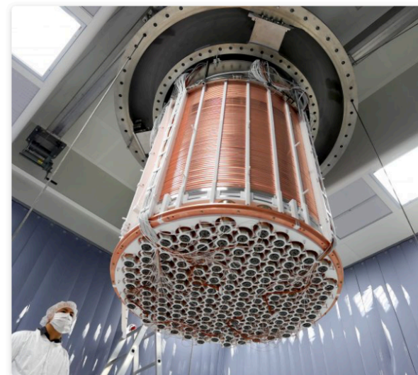
The XENON1T detector. Visible is the bottom array of photomultiplier tubes, and the copper structure that creates the electric drift field.
