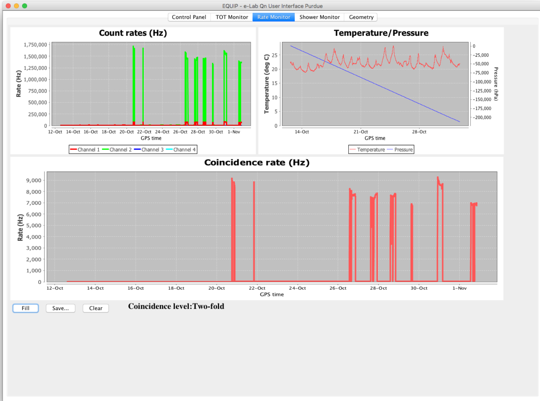
Fig 11: Vaughn detector data taken over 19 days in May-June, 2019 (the date axes are incorrectly labeled October, and the pressure sensor data is not right)
