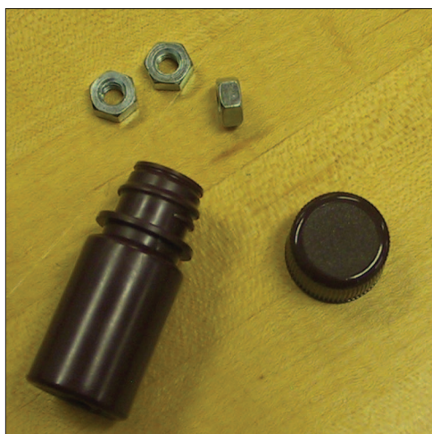
Fig. 1. Picture of one of the containers (the "oil drop") and the steel nuts (the "electrons").
